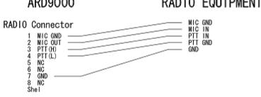
Note: MIC GND and GND must not be connected together in the ARD9000 connector, or RF feedback will result.
